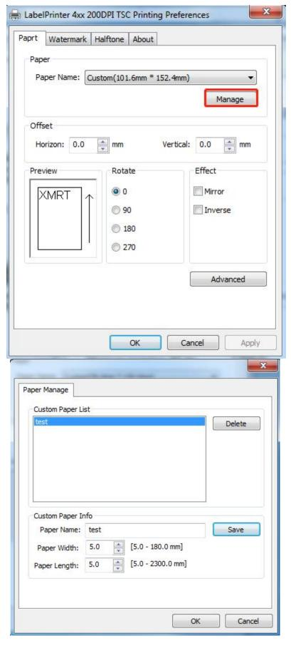
Offset sets horizontal and vertical margins. Rotate to print in different directions.
