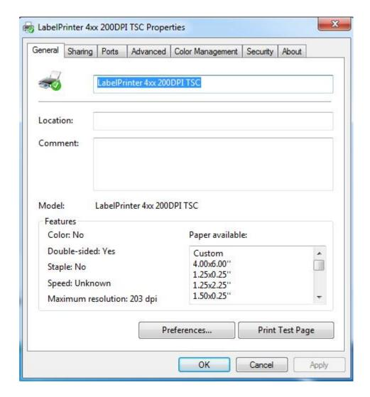
On Label Printer "General", you could configure the printer communication port, such as Serial port, Parallel port and USB port. You also could set the paper specification, beeper etc.
